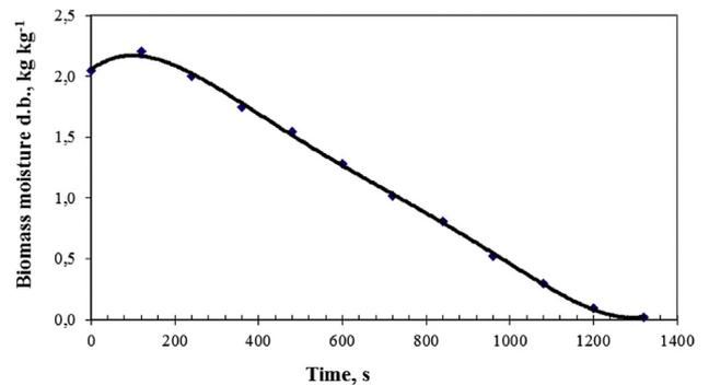
**Fig. 4 – Biomass drying curve in an agitated fluidised bed.**
