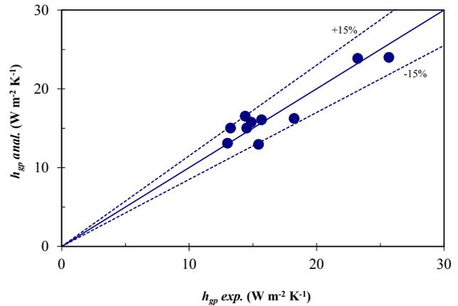
**Fig. 7 – Comparison of the experimental  $h_{gp}$  values with values calculated with the proposed correlation.**
