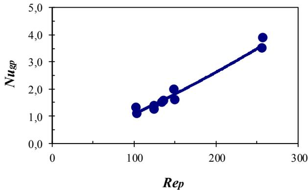
**Fig. 5 – Nusselt–Reynolds correlation for a forest biomass fluidised bed according to Eq. (10).  $R^2 = 0.9473$ .**
