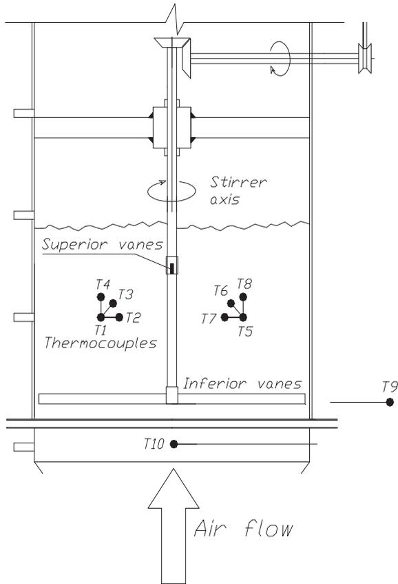
**Fig. 2 – Drying chamber with agitation system and temperature probes.**
