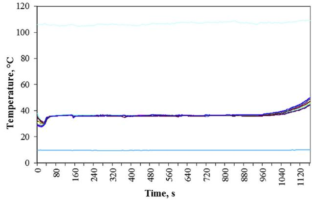
**Fig. 3 – Evolution of temperature at various locations in the bed during biomass drying in an agitated fluidised bed.**
